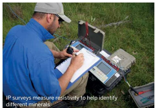
IP surveys measure resistivity to help identify different minerals
