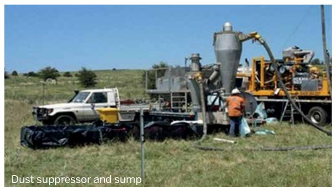
The handling of dust and spillages will depend on the particular dust suppression system used. Using black plastic beneath cyclones to catch spillage makes clean-up easier. Eliminating material falling on the ground significantly reduces the clean-up time and impact of the drilling.
